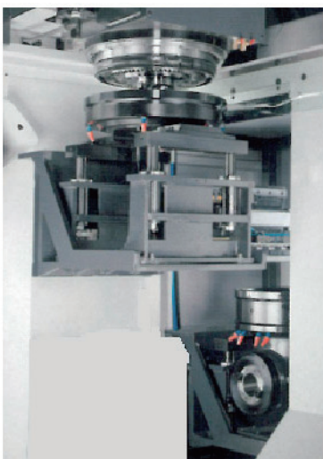
■ 1+1 Attachment system (one milling head change auto.)
